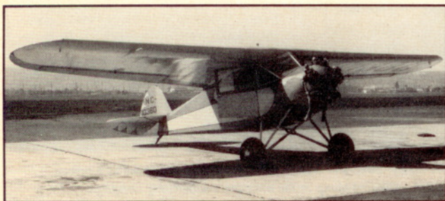
The Kari-Keen Coupe, the Sioux Coupe and finally the Swanson Coupe were all basically the same cantilever-wing cabin monoplane first designed by Swen Swanson. The Depression brought on their demise.
