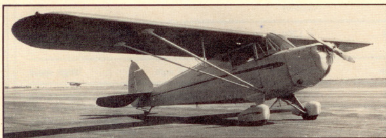
An early Ercoupe contemporary, the Piper J-4 Cub Coupe was basically the same airplane as the J-3 Cub but with a widened fuselage for side-by-side seating. The J-4E model was equipped with an enclosed 75-hp Continental A-75 engine.
