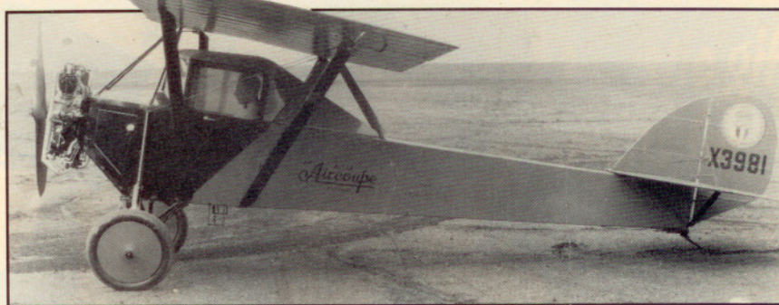
Essentially a two-seat parasol monoplane, the Elias Aircoupe fits the modern conception of a coupe-type airplane. A side door added to the fuselage earned the Aircoupe a genuine cabin.
